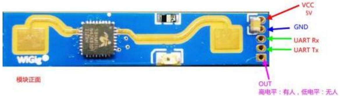
Figure 1 Module pin definition diagram
