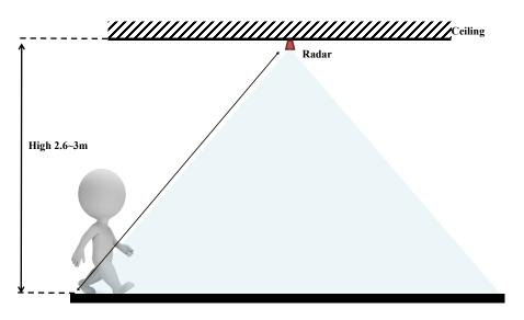
Figure 7 Schematic diagram of ceiling-mounted installation
