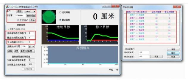
The ball is the target status output indication: red means there is a moving target; purple means there is a stationary target; green means no one.
