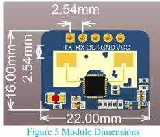
Module size: 16mmx22mm, 5 pin holes are reserved in the hardware (the factory default does not match the pins) The pin hole diameter is 0.9mm, and the pin spacing is 2.54mm.
