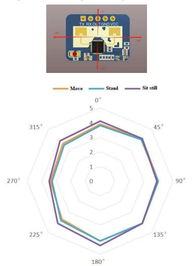
(distance unit: meters, angle unit: degrees) Figure 8 Schematic diagram of the detection range (the ceiling height is 3 meters)
