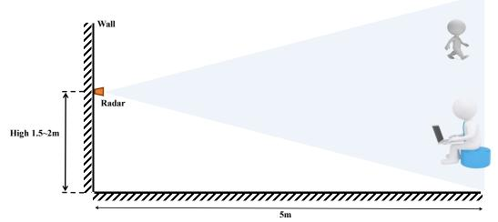
(distance unit: meters, angle unit: degrees) Figure 9 Schematic diagram of wall-mounted installation
