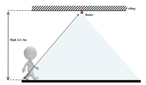
Figure 7 Schematic diagram of ceiling-mounted installation
