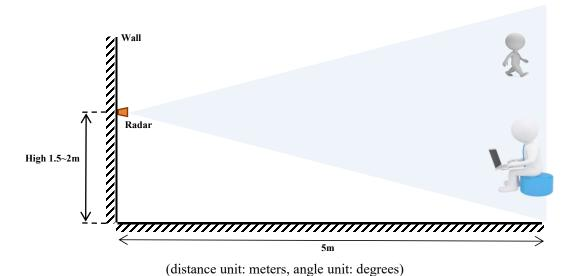
Figure 9 Schematic diagram of wall-mounted installation
