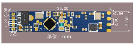
**Figure 5 Module Dimensions**
