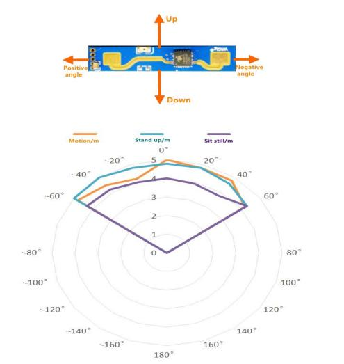
Figure 10 Schematic diagram of the detection range (the height of the wall is 1.5 meters)
