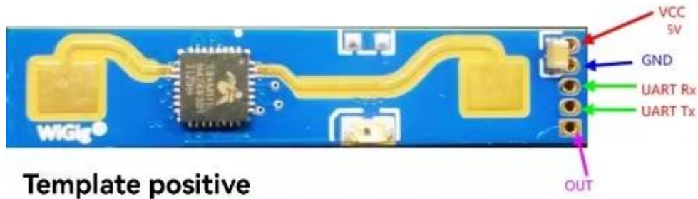
Figure 1 module pin definition diagram
