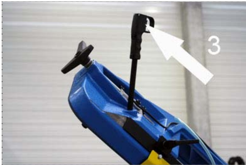
Fig. 5 – Start and stop control
