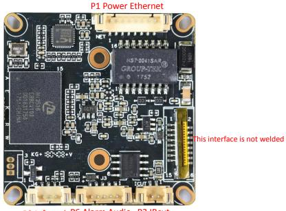
P3 Infrared P6 Alarm Audio P3 IRcut
