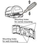
3) Install the detector on the bracket and connect the wires (see section 8).
